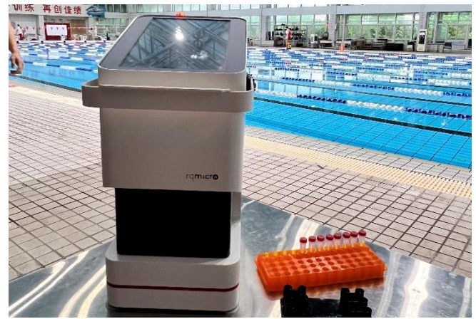
Performing analysis with the rqmicro.COUNT on-site at the swimming pool.
